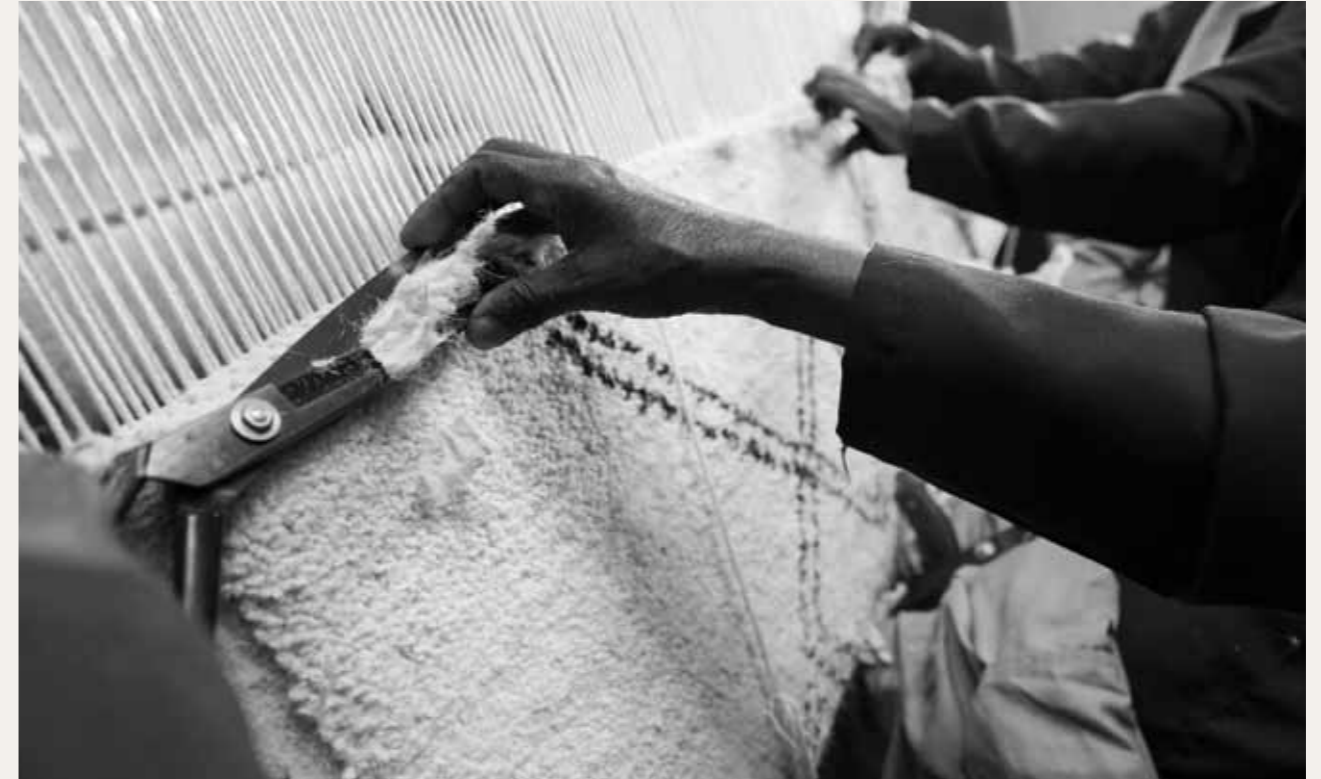
3. Cutting the correct height of the knots.
